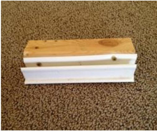
Figure D3. BTM Track with 2x2 base on pavement
