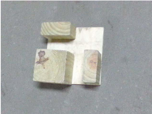
Figure E1. Landing framing jig.
